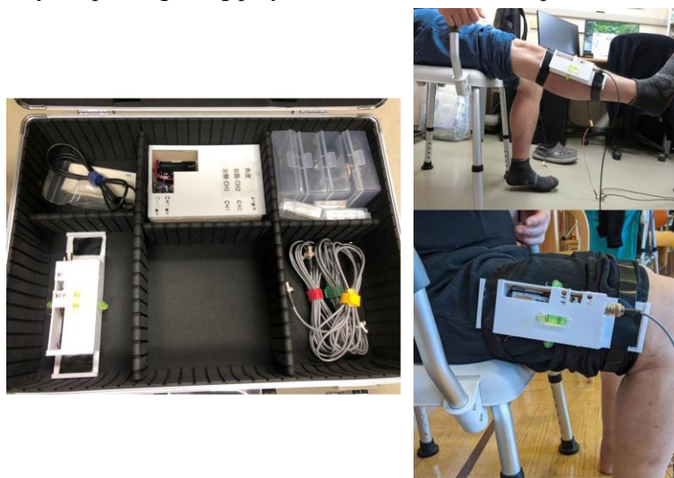
Figure 2.2.5 The VAG signal collection device developed in this study and bound to the participants.
