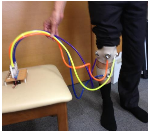
Figure 2.1.2 A view of the actual use of the knee joint sound collection device
