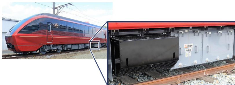
Fig.1.1. Power conversion circuit for rolling stock [3].
