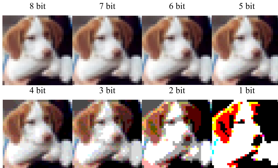
Figure 3.2: Example of linearly quantized images.
