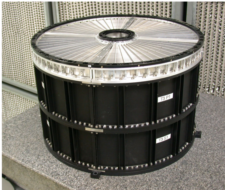
Fig. 4.8 XRT : X-ray mirror of Suzaku .
