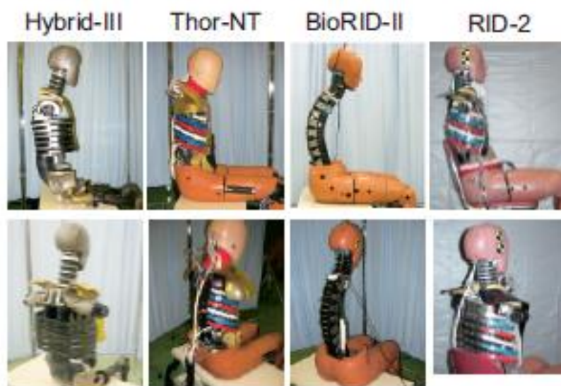
Fig. 2-9 Crash dummies for whiplash injury evaluation (Ministry of Land, Infrastructure, Transport and Tourism Automobile Transportation Bureau, 2005).
