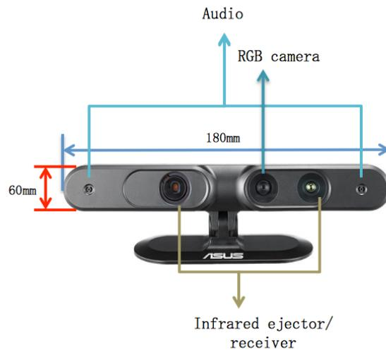
**Figure 3.4:** Profile of the Xtion sensor.
