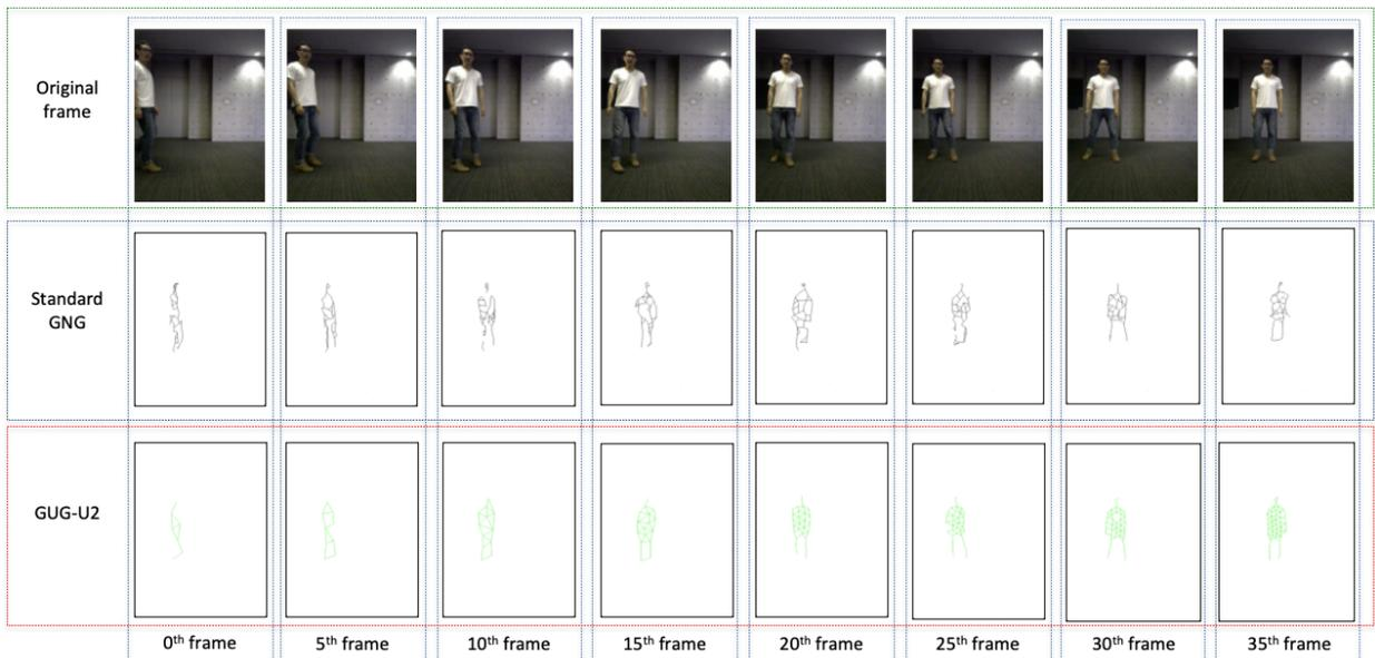
**Figure 3.6:** Experiment result between the standard GNG and the GNG-U2 in a series of input frames. The first row represents the original frame, the middle row shows the standard GNG, and the last row shows the GNG-U2.
