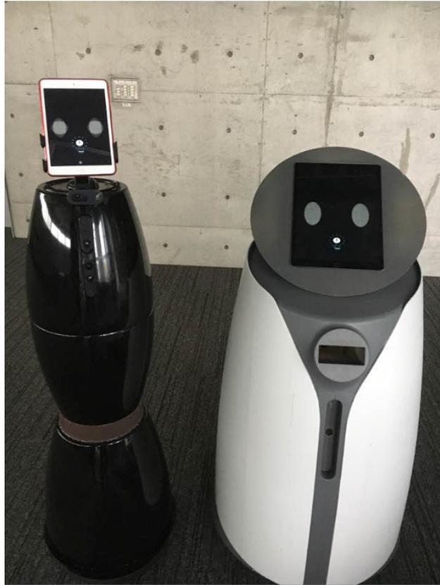
**Figure 5.16:** *Appearance of the airport robot. Left one is the prototype whereas right one is advanced designed shape.*
