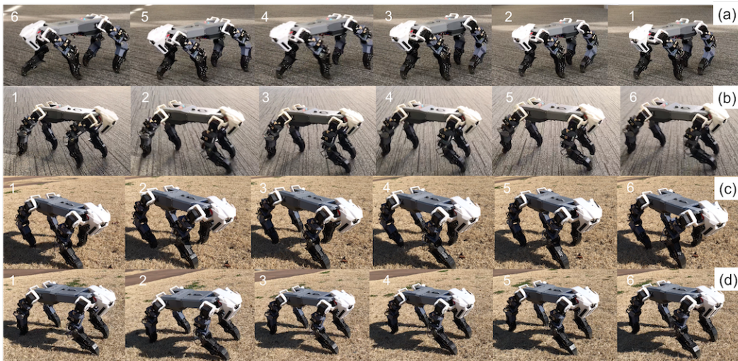
Figure 3.22: Snapshots of the robots performance shows the dynamic gait pattern during leg injury: a) the robots performance on the flat terrain with a forelimb injury; b) the robots performance on flat terrain with a hindlimb injury; c) the robots performance on natural terrain with a forelimb injury; d) the robots performance on natural terrain with a hindlimb injury.
