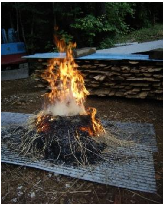
Figure 2.19. I burned rice straw ash for making glazes. Source: Andrew J. Gemrich Weblog
