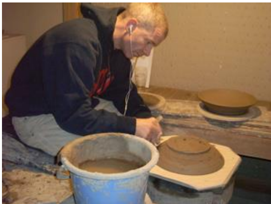
Figure 2.21. Trimming plates. Source: Andrew J. Gemrich Weblog
