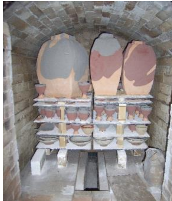
Figure 2.20. Glazed pieces in the kiln for firing. Source: Andrew J. Gemrich Weblog
