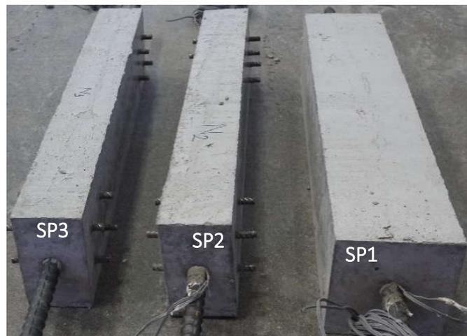
Figure 3-3: Substrate concrete specimen after casting
