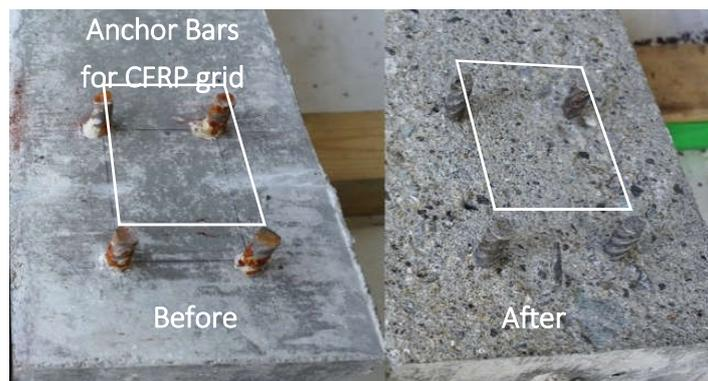
Figure 3-4: Concrete surface before and after sandblasting
