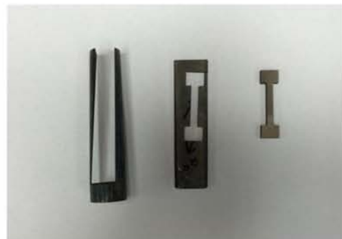
Fig.3.2 Shapes of specimen for creep test (a) Specimen geometry for tensile and compression test.
