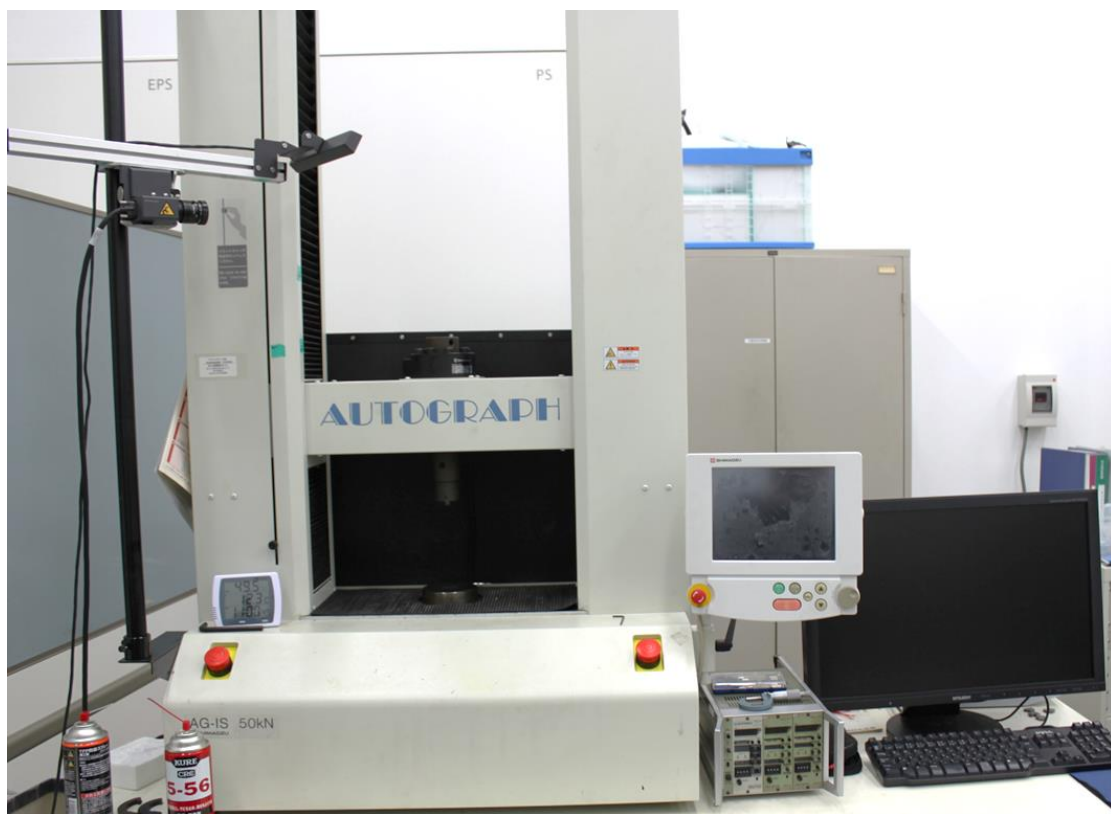
Fig. 3.4 titanium foam specimens were examined by compressive tests at room temperature using a Shimadzu Autograph AG-50kNISD.
