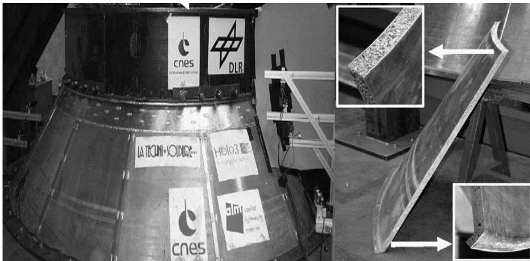
Fig. 1.4. Application of metal foam sandwich structure in the aerospace field.
