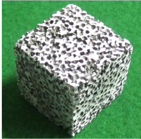
Fig. 1.8 The open cell AZ31 Mg alloy foam, sample with 1.70 mm \varnothing (30 mm*30 mm*30 mm).
