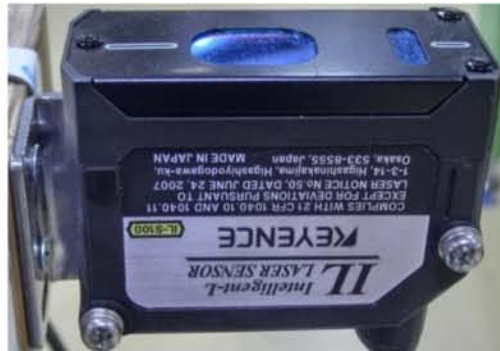
Fig. 4-6 Photograph of laser displacement meter
