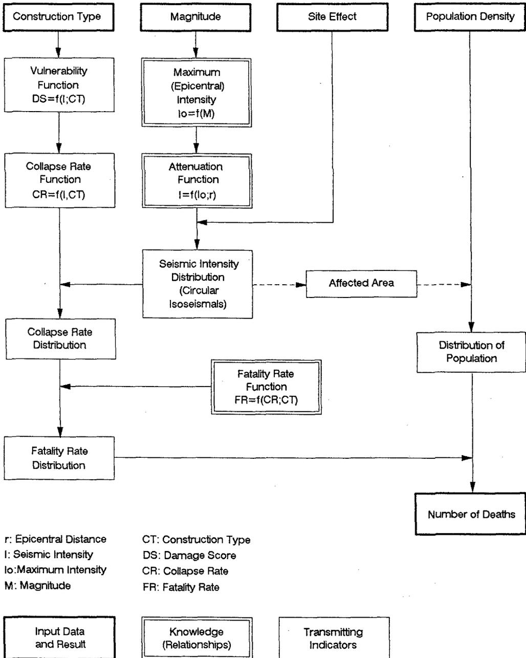
Figure 1. General structure of the model.
