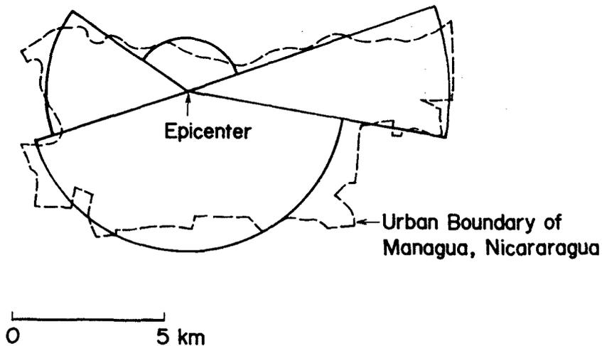
Figure 10. Segmentation of the affected area, Managua, Nicaragua for calculation.
