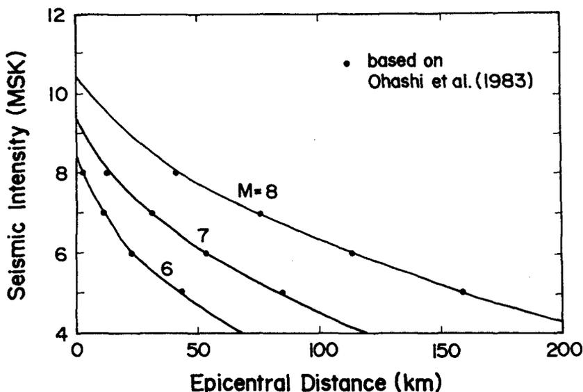
Figure 17. Attenuation curves of earthquakes in Turkey.
