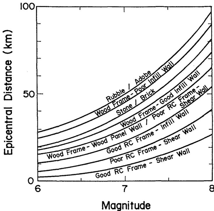
Figure 8. Epicentral distance within which building collapse and fatality are expected.
