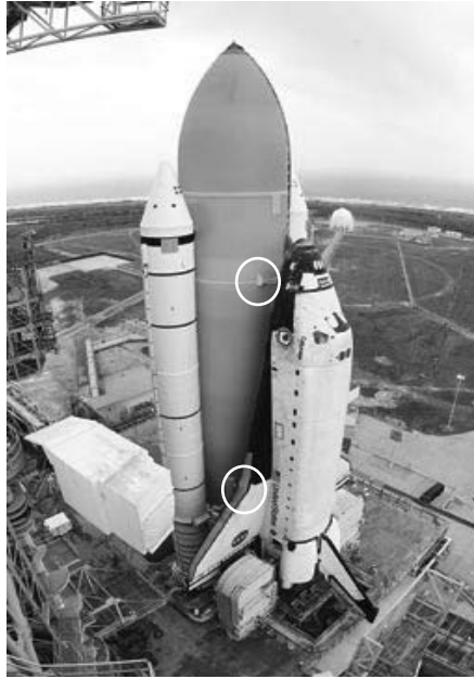
(a) Columbia sitting at Launch Complex 39-A. The upper circle shows the left bipod (-Y) ramp on the forward attach point, while the lower circle is around RCC panel 8-left.
