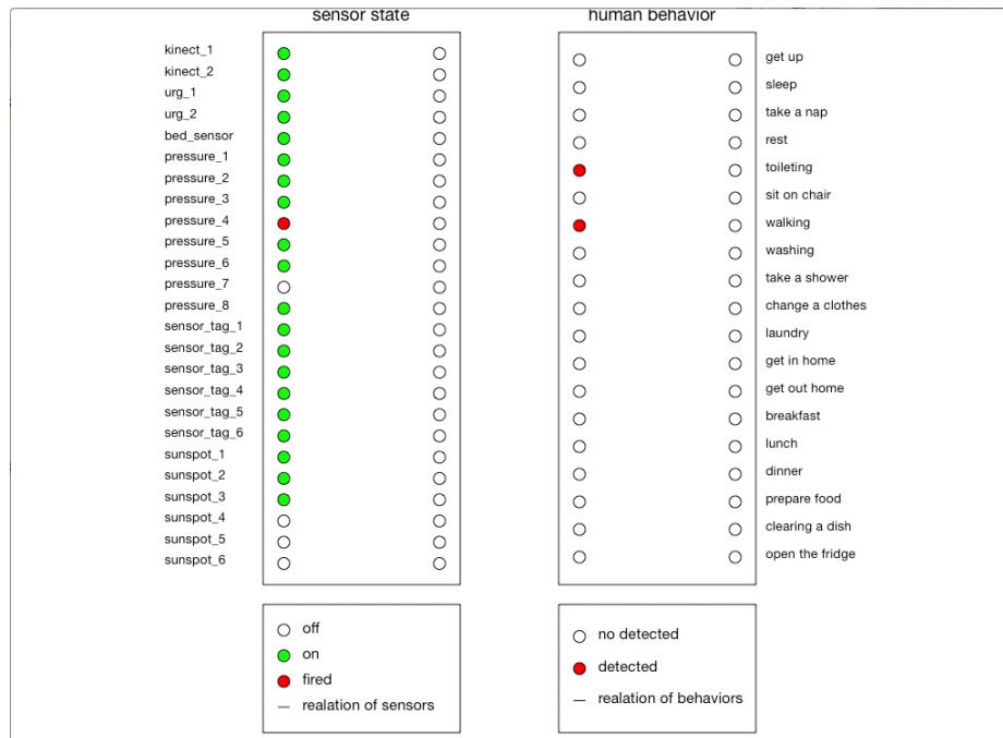
Figure 3.29: Fire states of sensors and behaviors
