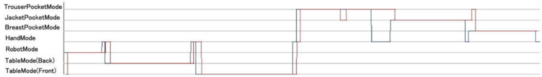
Figure 3.27: Experimental results by using FSNN for test dataset 2 after parameter optimization (using smoothing function in Eq. 3.9)
