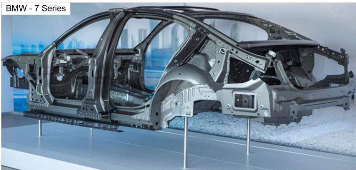
Figure 1.2. CFRP (the black portions) on body frame of BMW – 7 Series
