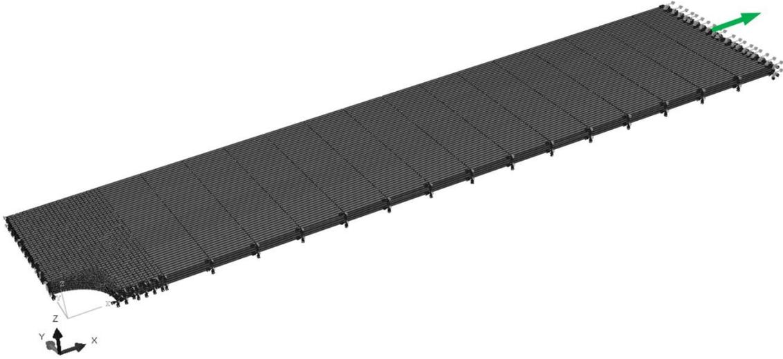
Figure A.2: Finite element model of open-hole tension test
