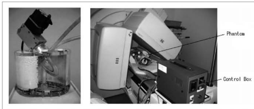
Fig. 4 Setting the dynamic cardiac phantom in gamma cameras. (a) Overview of the phantom. (b) Setting the phantom.
