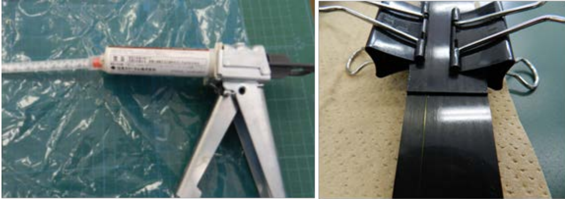
Figure 42 : Adhesive gun-mixer system and specimen pre-fit.
