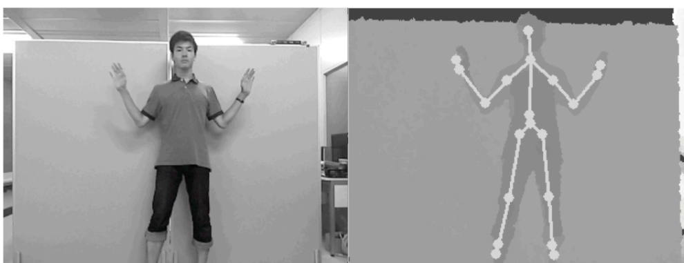
Fig. 4.39 Camera image and skeleton model measured by kinect sensor.
