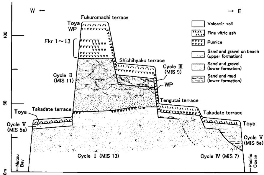
Fig. 6 Generalized section showing relationships between marine terraces and the marine Pleistocene from western to eastern parts of the central Kamikita Plain. Cycles II - V comprise marine terrace deposits of Fukuromachi, Shichihyaku, Tengutai, and Takadate. Noheji formation is composed of cycles I, II, and IV which are the basements under marine terraces.
