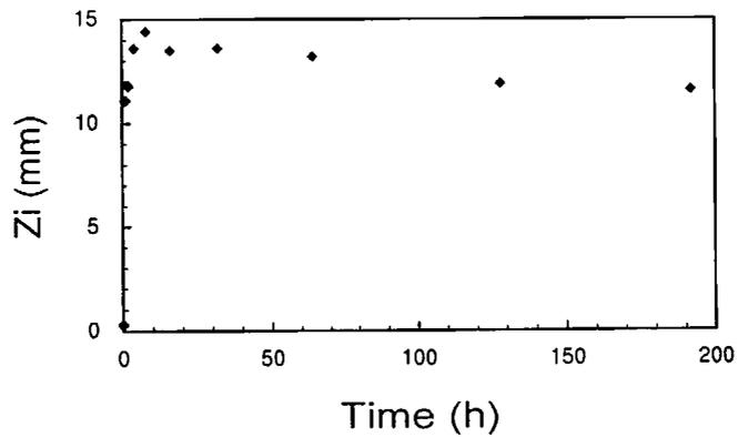
**Fig. 2** Changes of the average standard deviation of elevation in a  $10 \times 10$  cm square,  $Z_i$ , with time
