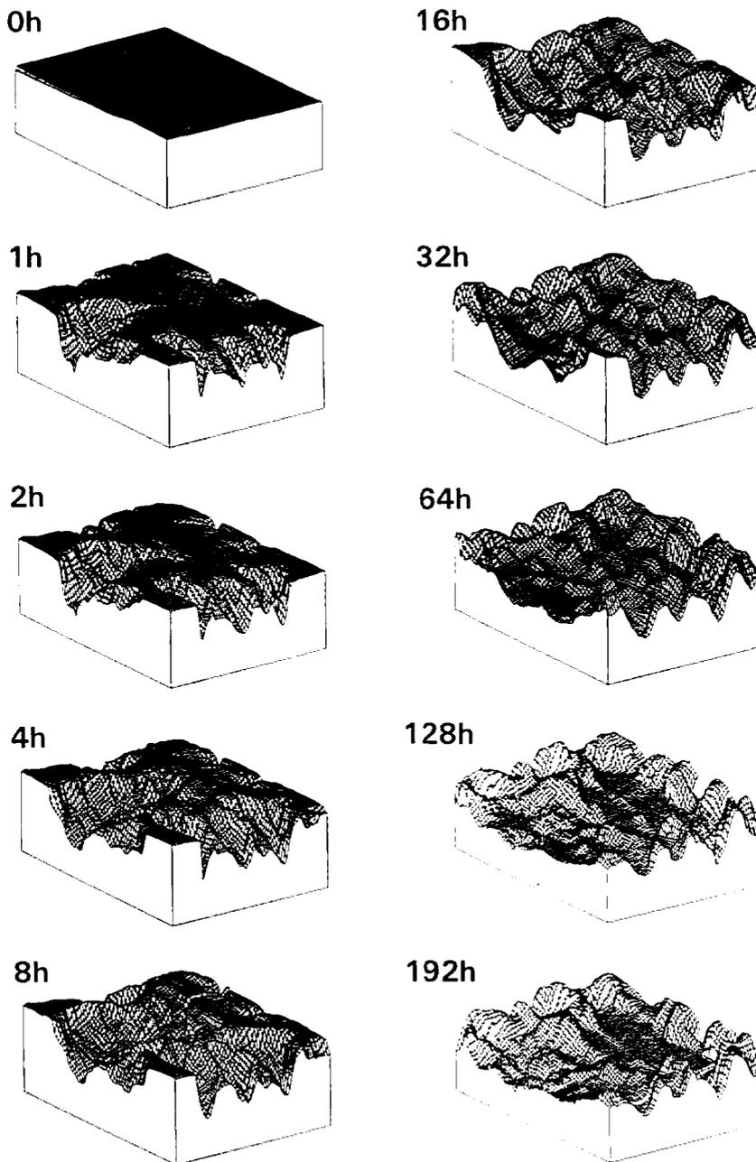
**Fig. 1** Block diagrams showing the changes of surface topography of the mound with the time of artificial rainfall application
