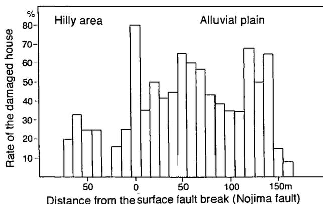
Fig. 3 Relationship between rate of damaged houses and distance from the surface fault rupture in Toshima, northwestern Awajishima (after Minagawa *et al.*, 1995)
