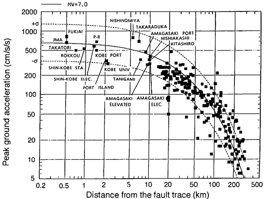
Fig. 5 Relationship between the observed peak acceleration and the distance of observation points from the active fault
