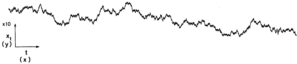
Fig. 2 An example of one-dimensional random walk (Brownian motion) trace X_t \sim T^H ( H=0.5 ). And X_t \sim N^{\nu_{xt}} ; T \sim N^{\nu_t} , when the two coordinates are scaled differently ( H = \nu_{xt}/\nu_t ).
