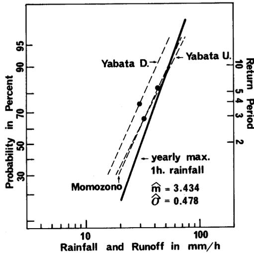
Fig. 4 Cumulated probability function of yearly maximum 1 hour rainfall and the corresponded runoff derived by eq. (14)
