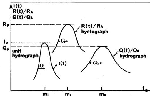
Fig. 1 Schematic diagrams of unit hydrograph, hyetograph and hydrograph
