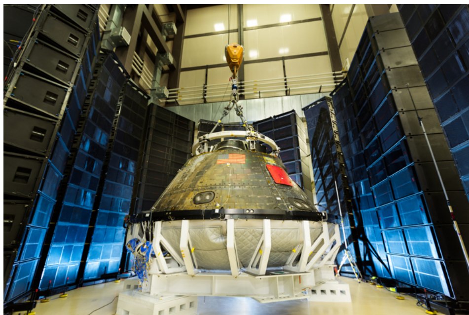
Figure 2-1. The overview of the DFAT for the Orion Spacecraft ©Dusty Volkel/Lockheed Martin
