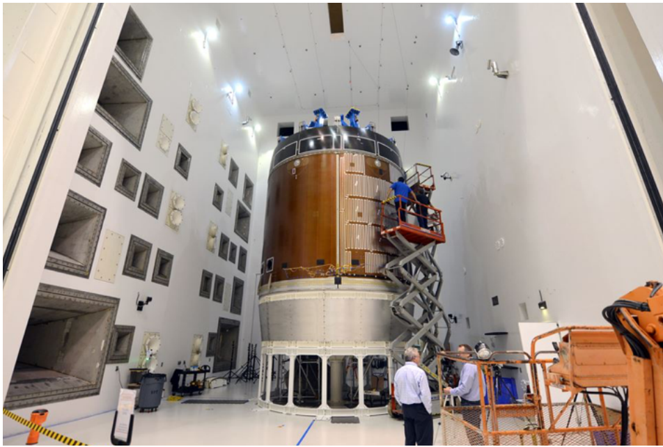
Figure 1-6. The overview of the NASA's Reverberant Acoustic Test Facility ©Jason Werling/NASA
