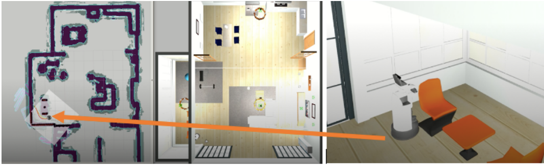
Figure 3.12: The example results in failed navigation behavior using the predicted map and TEB Planners. The other planners also failed in this stage. The predicted map could not predict this type of chair. The leg part of the chair has a flat surface that is adhered to the floor.
