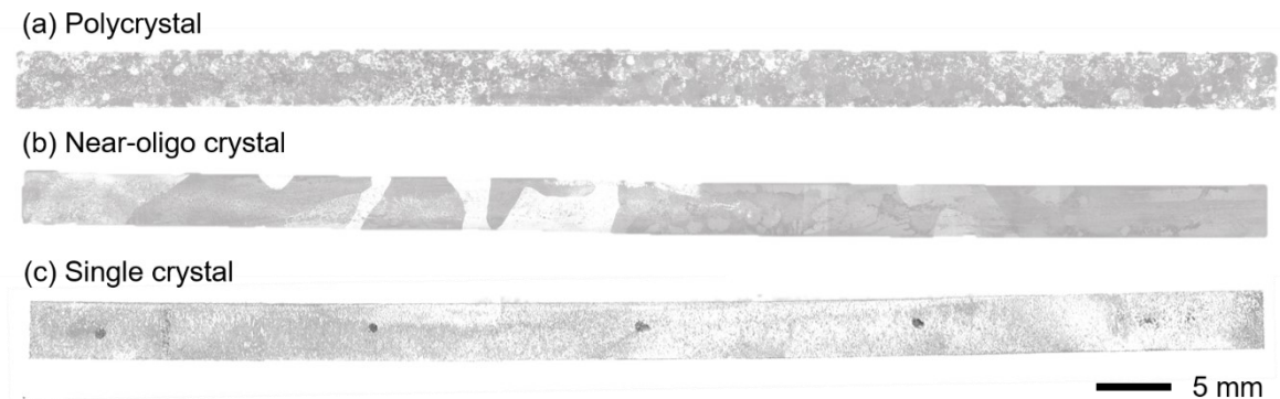
Fig. 4.2.2.1 Optical photos of (a) polycrystalline, (b) near-oligo crystal and (c) single-crystal Cu-Al-Mn SMA samples prepared for axial bending.
