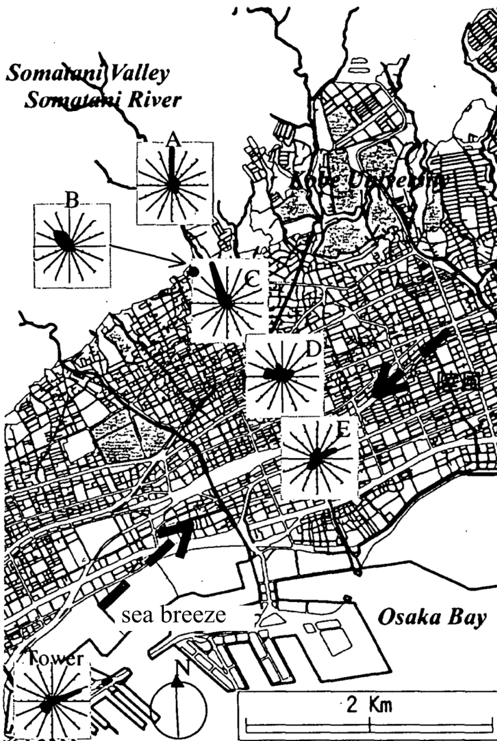
Fig. 1-14 Windrose at night for weak extended sea and land breeze (July 25-26, 1999 at 18:00 and 16:00 JST) The largest scale on the windrose is the 50% frequency (Takebayashi et al. , 2001).
