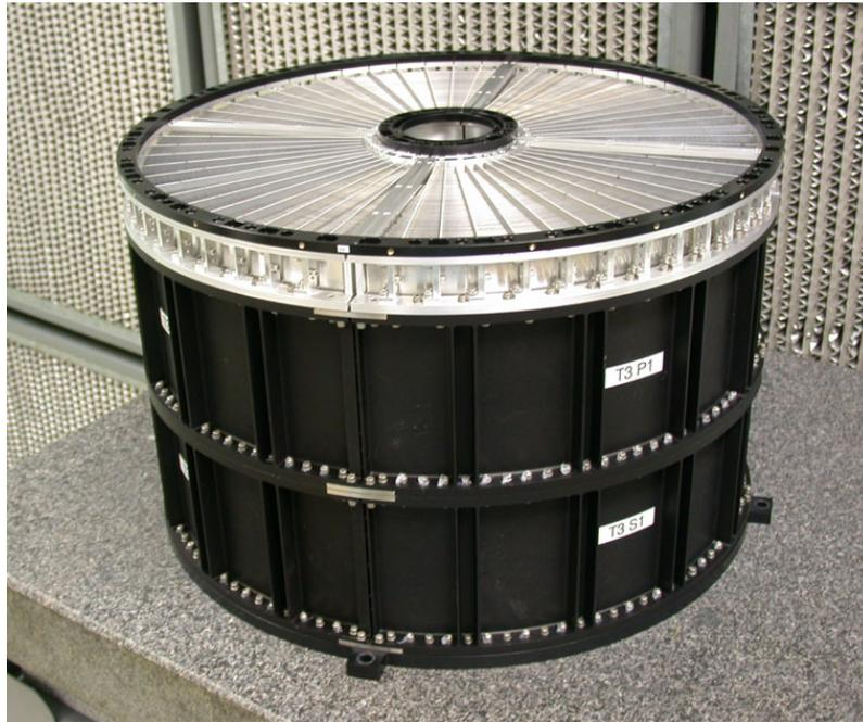
FIGURE 3.8: Photograph of *Suzaku's* X-Ray Telescope (XRT). Credit: NASA/GSFC
