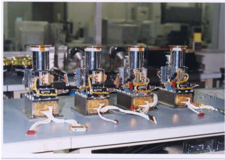
FIGURE 3.11: Photograph of the four X-ray Imaging Spectrometer (XIS) before installation onto *Suzaku*. Credit: NASA/GSFC
