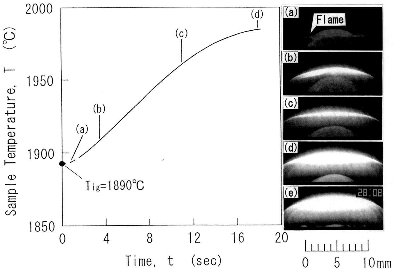
Fig. 2. Time variation of sample temperature and special video photographs in an  $\text{O}_2/\text{N}_2$  stream.
