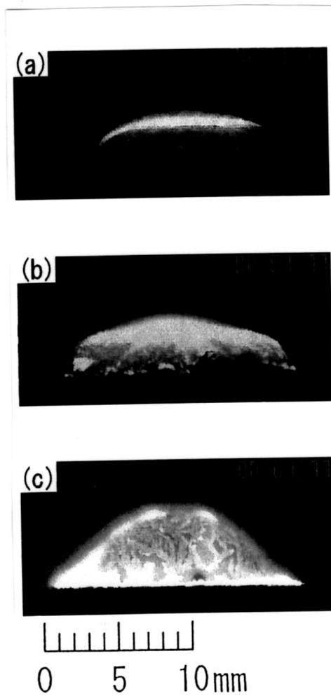
Fig. 5. Variation of flame height with  $X_{O_2}$  at 1.77 sec after ignition.
