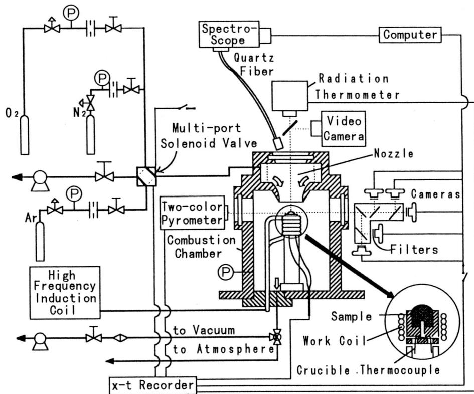
Fig. 1. Schematic of experimental apparatus.
