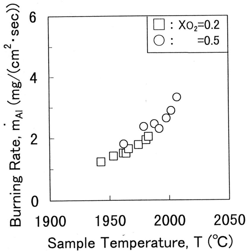
Fig.7. Variation of burning rate with the sample temperature.
