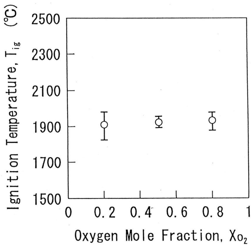
Fig. 3. Variation of ignition temperature with  $X_{O_2}$ .
