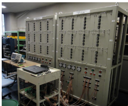
図 1.2 Photo of the three-phase 200-V, 10-kW, 50-Hz experimental system. 文献 [3] より引用
